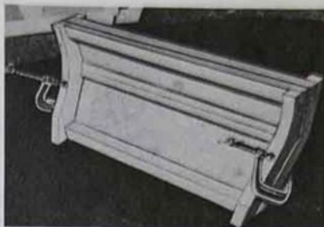
The critical joint between the bow bulkhead and the rear bulkhead of the locker must be a perfect fit. Fabricate both bulkheads in one operation
